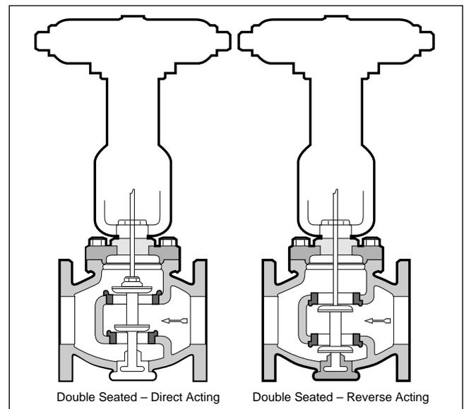
**FIGURE 12 - Double Seated Valves, Reverse/Direct Action**
