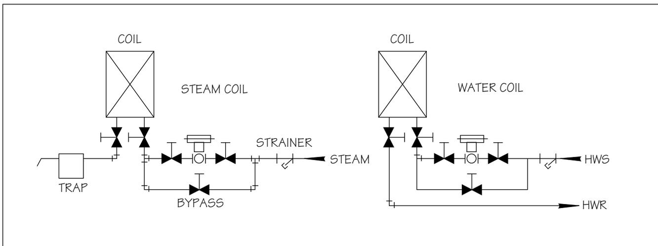
FIGURE 4- 2-way Valve Piping
