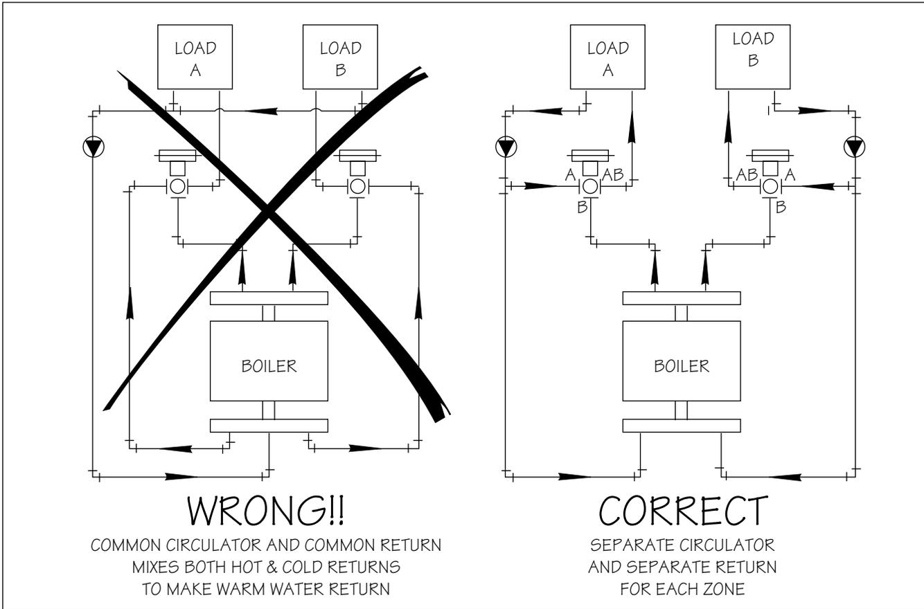
**FIGURE 8- Common Piping Errors**
