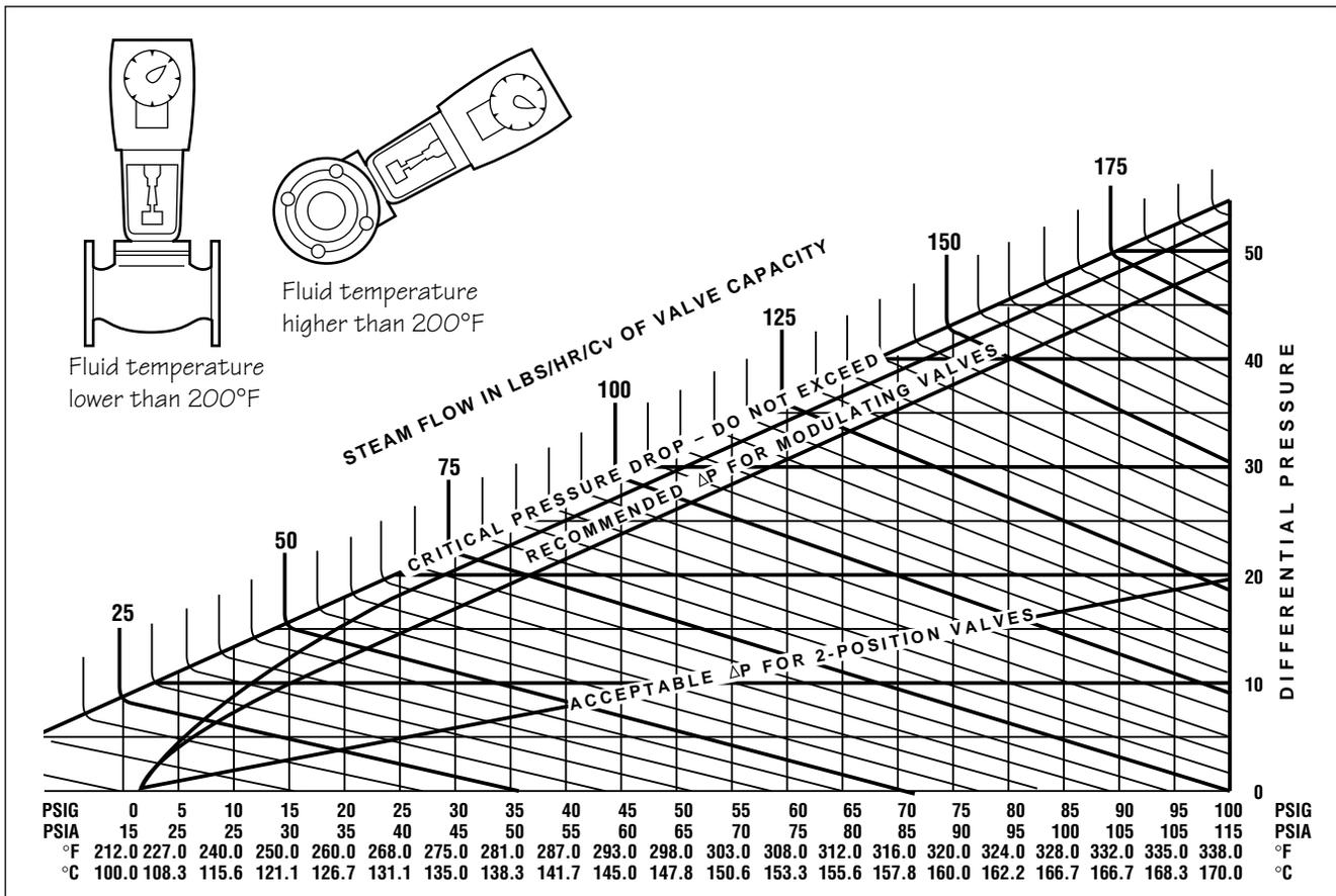
FIGURE 3 - Steam Valve Sizing
