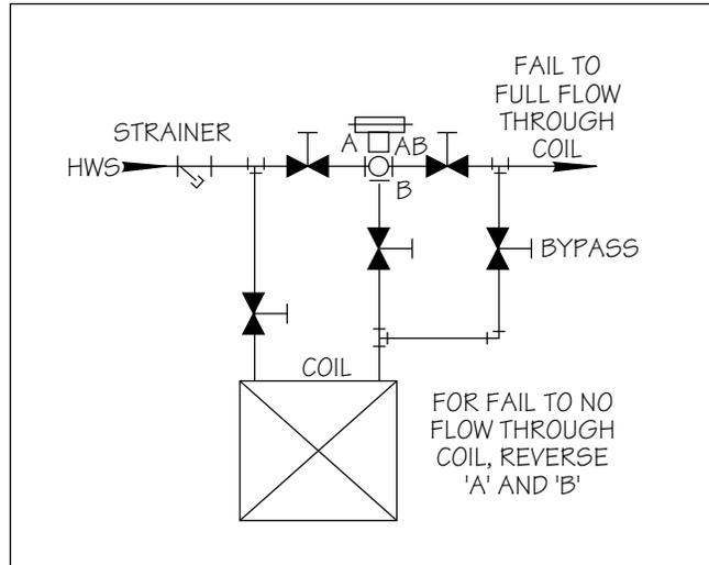
FIGURE 6 - 3-way Valve Piping
