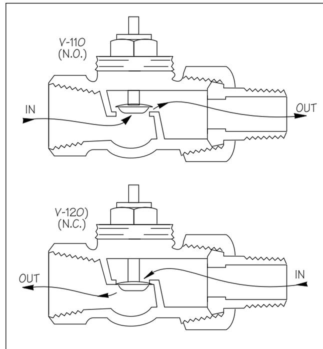
FIGURE 5 - V-11 (N.O.) & V-12 (N.C.) Valve Bodies
