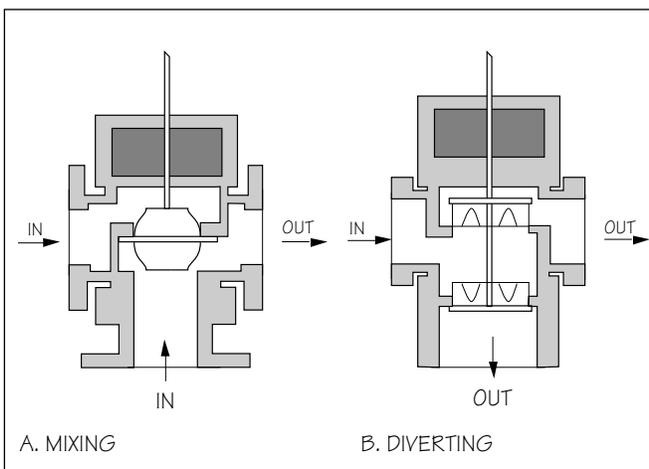
**FIGURE 11 - Typical 3-way mixing & diverting valves**
