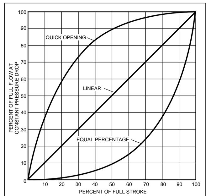
**FIGURE 13 - ASHRAE Valve Characteristics Graph**
