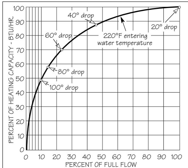
See **Figure 1** which plots the heat output of a coil vs flow.
