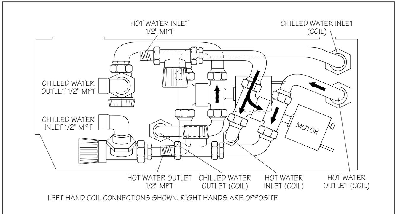
FIGURE 14 -View from Side of a Typical Fan Coil Unit.
