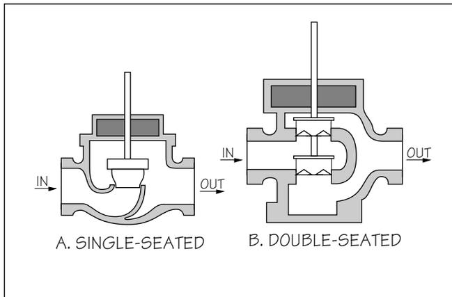
**FIGURE 10 - Typical single- & double-seated valves**
