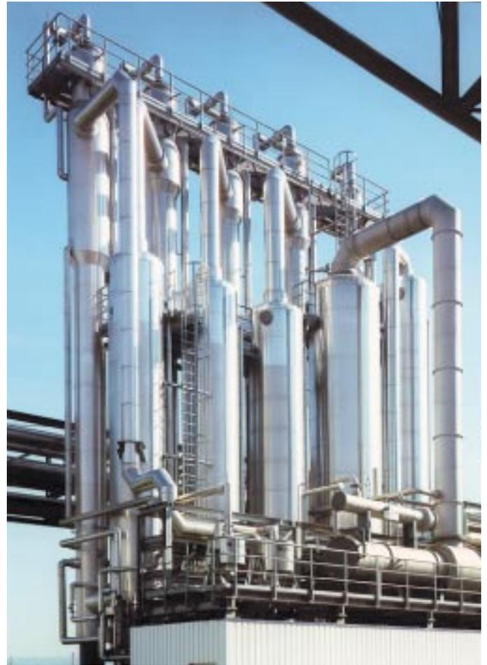
**Right:** A 4-effect, continuous rectification plant with falling film reboilers, downstream finisher and residue concentration system, designed for process water from the production of hollow fibre modules
